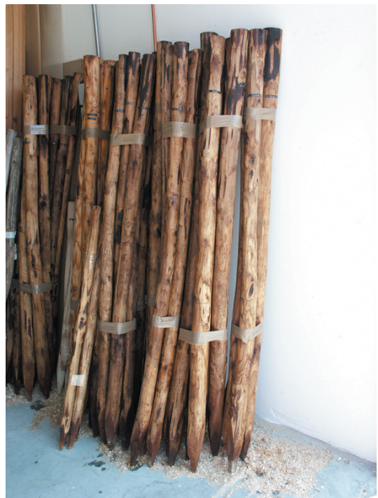
Figure 3: chestnut poles treated with hot linseed oil.
