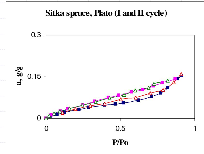
I cycle adsorption (■) and desorption (■), II cycle adsorption (△) and desorption (△).
